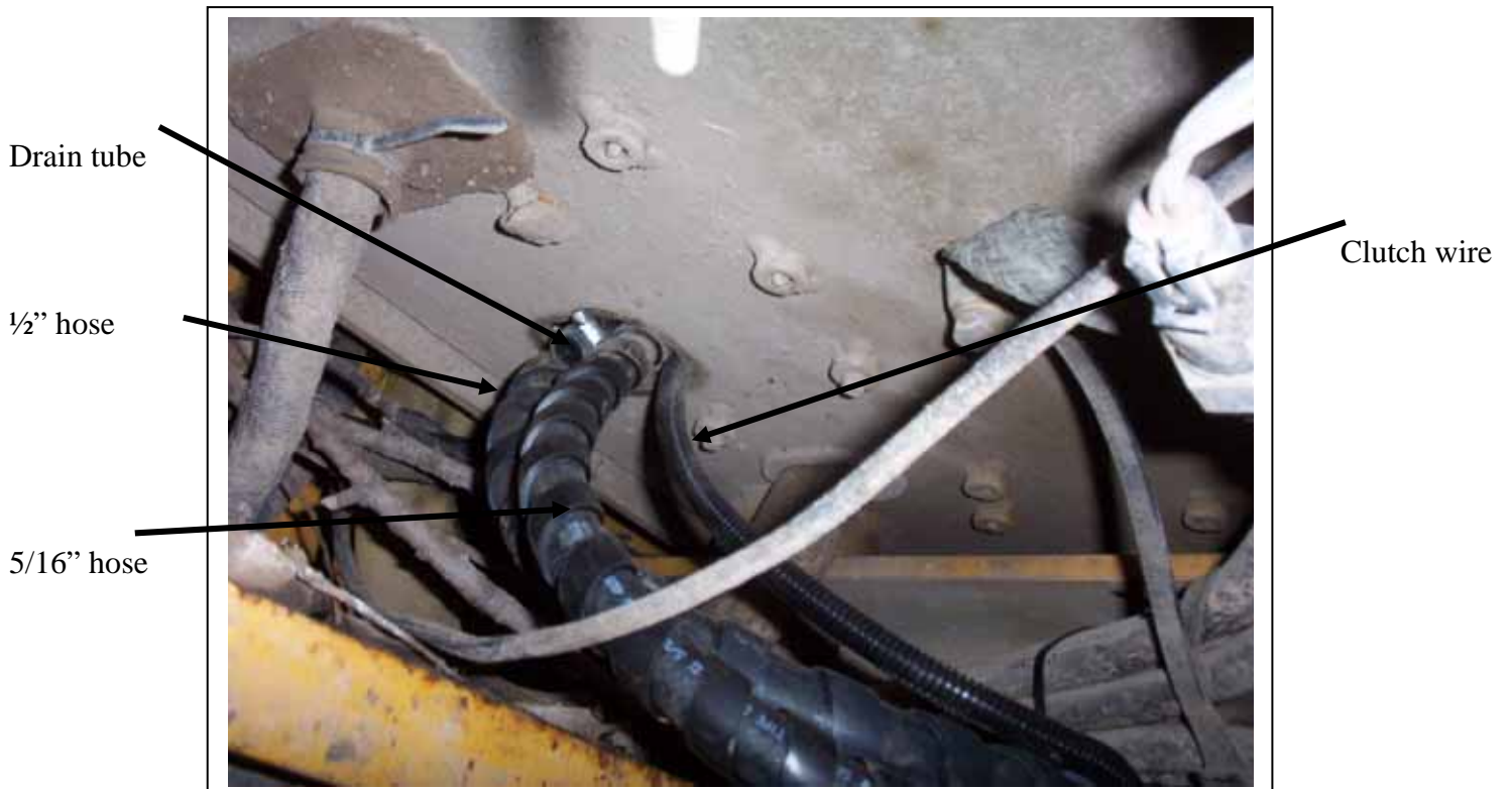
A/C hoses, clutch wire and drain tube exiting the cab. View from under cab floor.
