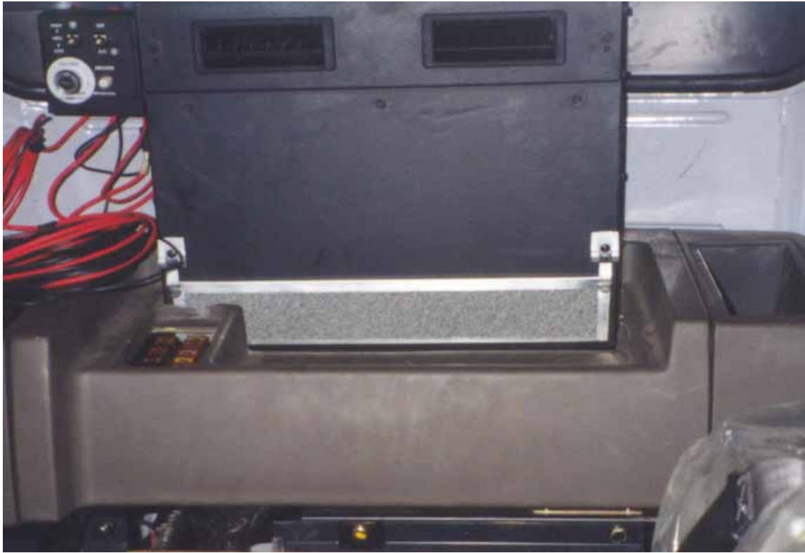
Evaporator in place on back wall of cab. Note that it extends above the lower window line.
