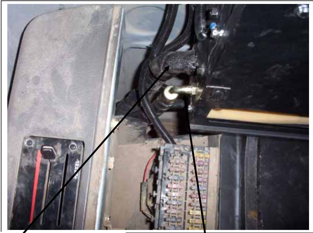
1/2" 90° male fitting at expansion valve.
